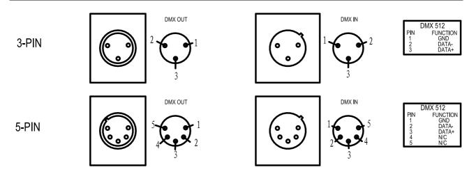
Connection between controller and projector and between one projector and another must be made with a 2 core-screened cable, with each core having at least a 0.5mm diameter. Connection to and from the projector is via cannon 5 pin (which are included with the projector) or 3 pin XLR plugs and sockets. The XLR's are connected as shown in the figure above.
