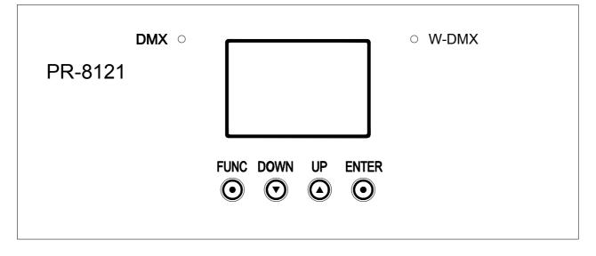
Projector configuration can be set conveniently via press button switch and LCD display.
