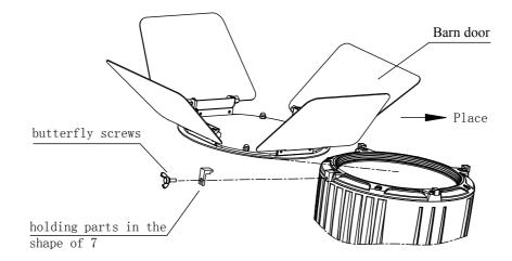
If the frost panel is also selected, it must be used in combination of the barn door. Its Installation and Dismantlement is illustrated in the diagrams below:
