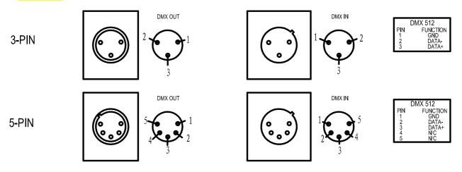
Connection between controller and projector and between one projector and another must be made with a twin-screened cable, with each wire having at least a 0.5mm in diameter. Connection to and from the projector is via cannon 5 pin (which are included with the projector) or 5 pin XLR plugs and sockets. The XLR's are connected as shown in the figure above.
