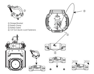
Regardless of the rigging option you choose for your MINI BEAM 1R, always be sure to secure your fixture with a safety cable. The fixture provides a built-in rigging point for a safety cable on the hanging bracket as illustrated above. Be sure to only use the designated rigging point for the safety cable and never secure a safety cable to a carrying handle.
