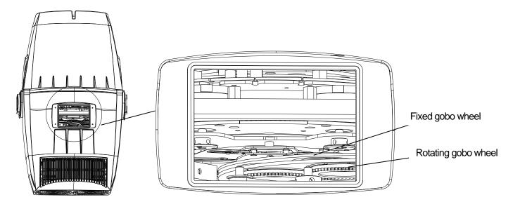
Lock the tilt and loosen the 4 fast-fit screws on the upper cover, After removing the cover, you will see the structures as the figure above.
