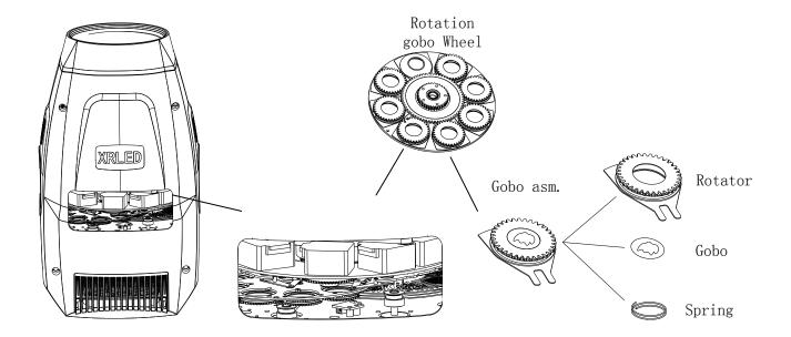
Open the head cover after locking the Tilt and loosening 6 fast-fit screws of the cover and the structures as illustrated by the above figures will be seen.
