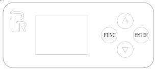
Fixture's address and function code configuration can be set conveniently via Touch Key and LCD display. Press button ENTER more than 3 seconds to unlock panel. LED display shows the fixture's function menu. Each Option of the main menu has its own sub-menu. Each menu stands for specified function of the fixture, please see the details in the following:
