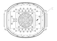
Figure 1: After loosening the 4 screws marked as A,B,C,D, remove the cover at the lamp end of the head. Pull the fan assembly after loosening the screw marked as E and the lamp chamber exposed.
