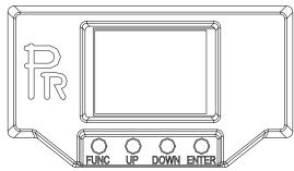
To browse through or change the projector 's settings, press ENTER key for more than 3s(press ENTER key after power on) to unlock the screen, then press UP/DOWN key to enter the projector 's function menus. Each main menu has its sub-menus. And each menu stands for special function. For the details, please see the following 6<sup>th</sup> point "Operation Menu"::
