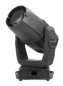
AQUA 580 BEAM is an all weather fixture having high optical efficacy ,low noise and multiple functions with ingress protection up to IP66. Front lens of 230mm produces full and solid beam with luminous flux of 230,000lux at 20 meters and beam angle at 2°. The fixture can project up to 500m like a strong searchlight with excellent in-air visual effects. Fast frost filter makes wash effects; 3 prisms make more fantastic and plenty in-air dynamic effects.
