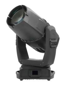
AQUA 580S BEAM is an all weather fixture having high optical efficacy, low noise and multiple functions with ingress protection up to IP66. Front lens of 230mm produces full and solid beam with luminous flux of 230,000lux at 20 meters and beam angle at 2°. The fixture can project up to 500m like a strong searchlight with excellent in-air visual effects. Fast frost filter makes wash effects.
